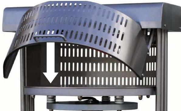
If the first start the bottom plate is not lifted completely, but rises only about 2 cm, the phase sequence is not correct. Reverse 2 phases on the power plug.
