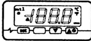
The thermostat starts automatically when the switch (A) is turned on. During normal operation the display will show the temperature of the plate. To set the thermostat, press the set button: the Led out 1 will flash. Within 15 seconds, press the buttons ▲ (up) or ▼ (down) and set the desired temperature of the plate. Once the desired temperature is set press set or press nothing for 15 seconds.
